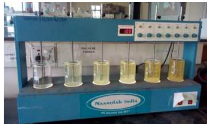
Fig - 6 Jar Test Using Natural Coagulant TRIGONELLA FOENUM – GRAECUM (Fenugreek Seeds)
