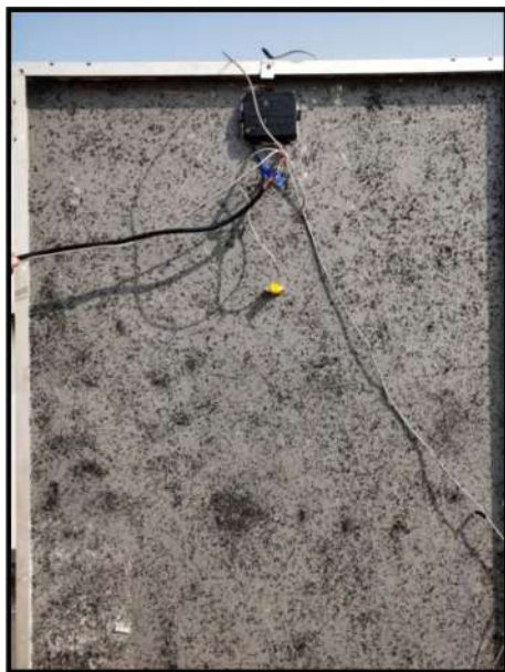
Fig. 3 Thermal grease and M.S chips applied on the backside of the PV panel
